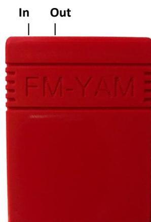
The FM-YAM has two audio sockets. One for **audio in** and another for **audio out**. See the picture to the left. Any **audio in** will be mixed by the output of the OPL2 (YM3812) music chip inside.
